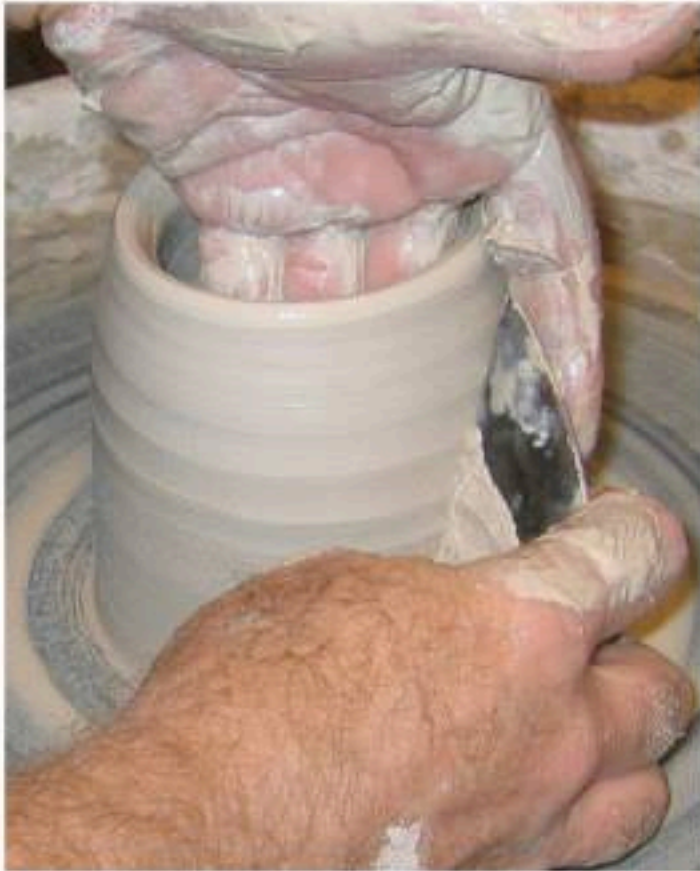
1. Throw a cylinder, scrape the sides clean with a rib
